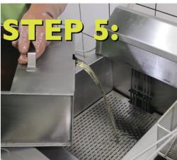
Fill the fryer with oil and set the thermostat to operating temperature.
