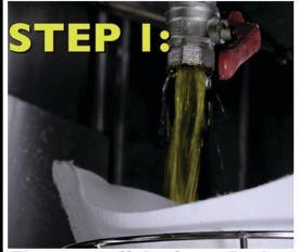
First turn off the fryer. Drain all the oil from the fryer in the normal way.
