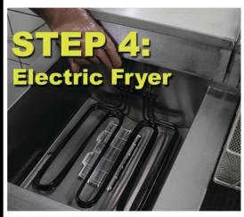
Option 2: Place Frylow under heating elements at the bottom of the fryer.
