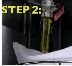
Turn fryer off and drain the oil in the normal way. Only install Frylow in an empty fryer.
